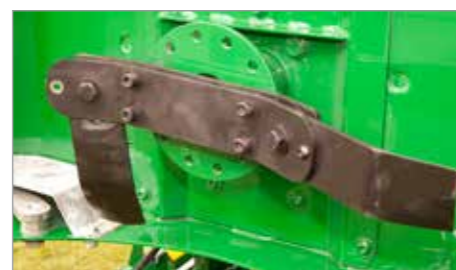
Two in one blade system, rigid and swinging
