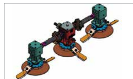
Synergy driveline and blade configuration
