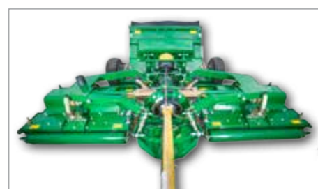
Robust frame with a centre pivot point and spherical bearings on the wings
