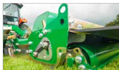
Cutting height adjustment system from 10 - 110mm
