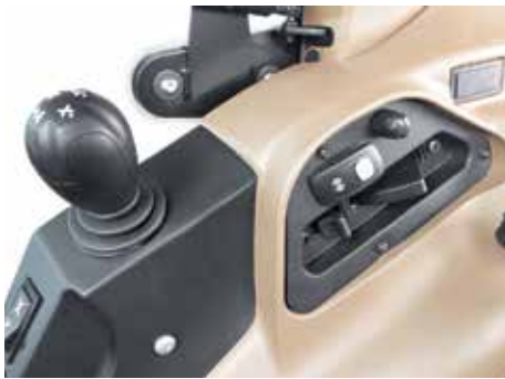
The mechanical hitch system features an easy to use quick raise and lower control.
