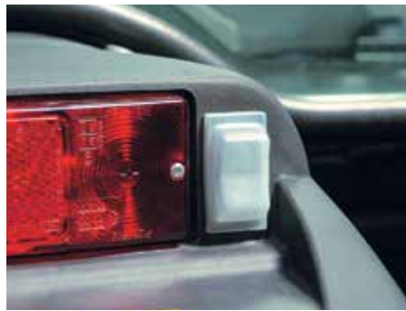
Fender-mounted hitch controls allow safe and easy attachment of machines and implements, even when working on your own.
