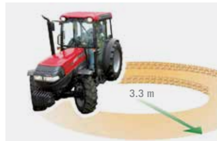
Turning radius of 3.34 m (Quantum 65V - 85V/F) and 3.44 m (Quantum 95 and 105 V/N/F).
